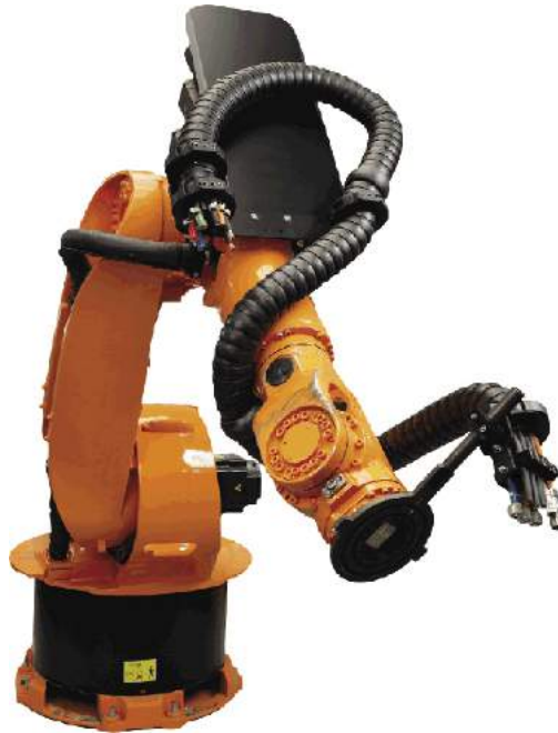
Figure 16: Cabel channelization on the Robot
