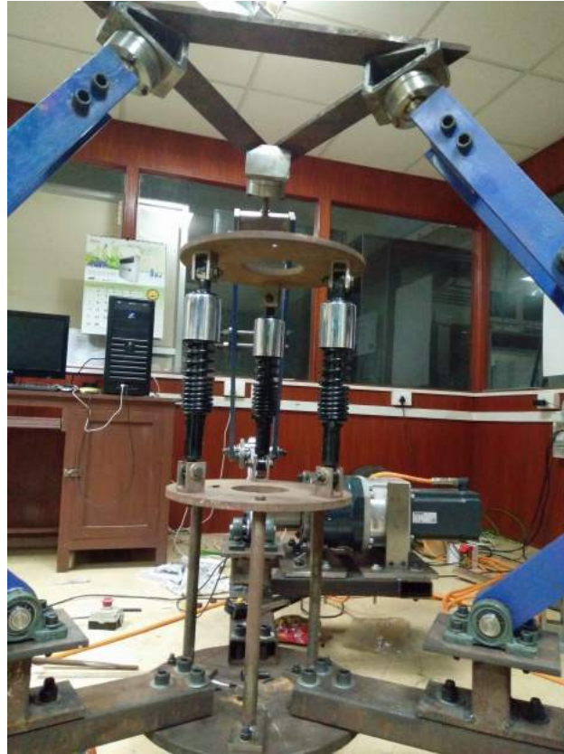
Figure 7: Shock Absorber for safe landing of the operator
