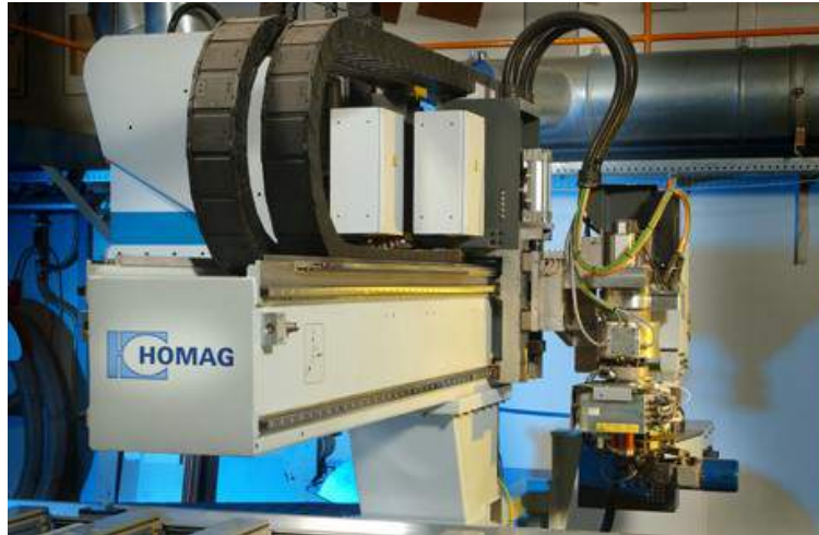
Figure 17: Drag chain on the machine
